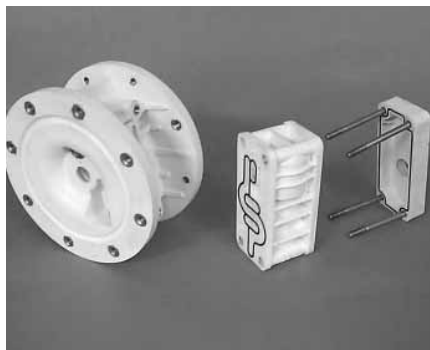
Step 2. Figure 2 Remove muffer plate and air valve bolts from air valve assembly exposing muffer gasket for inspection. Replace if necessary.
