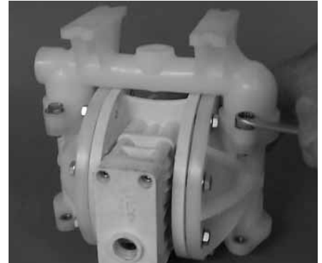
Step 5. Figure 5 Using a 1/2" box wrench, remove the inlet manifold.
