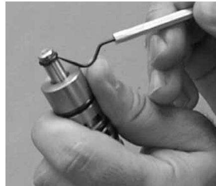
Step 8. Figure 8 With o-ring pick, gently remove the o-ring from the opposite side of the “center hole” cut on the spool. Gently remove the pilot spool from sleeve and inspect for nicks or gouges and other signs of wear. Replace pilot sleeve assembly or outer sleeve o-rings if necessary. During re-assembly never insert the pilot spool into the sleeve with the “center cut” side first, this end incorporates the urethane o-ring and will be damaged as it slides over the ports cut in the sleeve.
