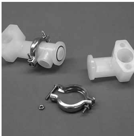
Step 7. Figure 7 Inspect o-rings for wear or damage and replace if necessary. PTFE o-rings should be replaced when reassembled.
